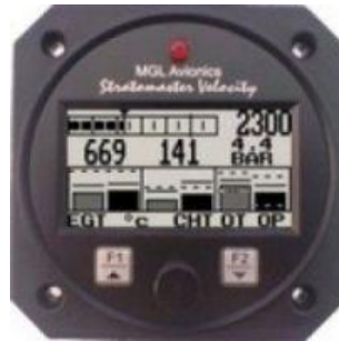
Example: the most common and convenient engine monitor MGL E1/E3
